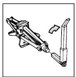
2. Attach the wheel wrench to the jack bolt head and rotate the wheel wrench clockwise. That will raise the lift head a little.
